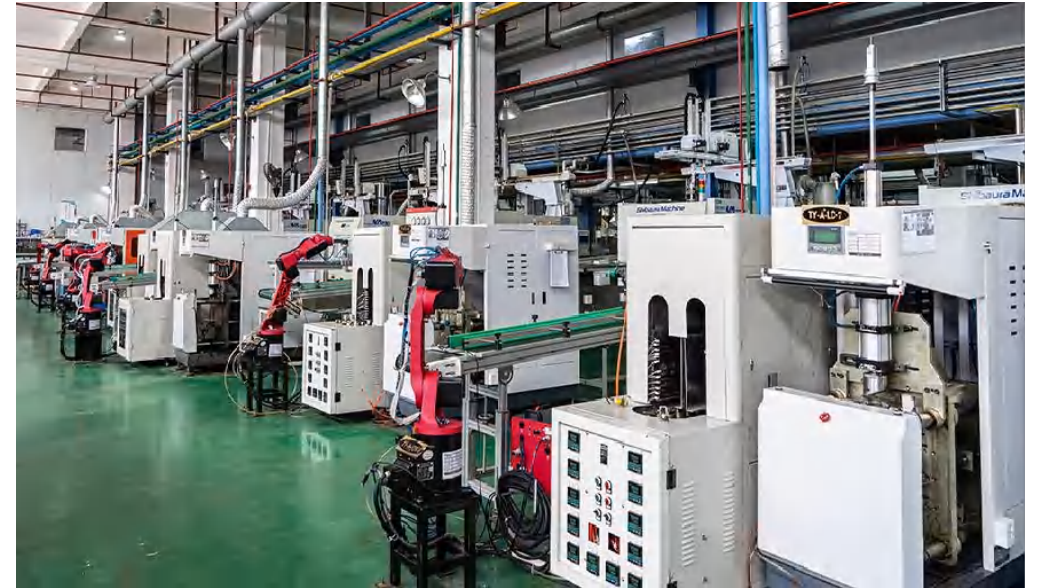
● Injection Stretch Blow Two - Step Process, Equipped with Electric Injection Molding Machines and Six - Axis Robots
